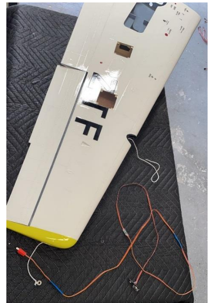
Above: weight on thread tip to pass the wires and wire to pull the wing landing light boards.
