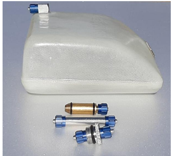
Above: fuel tank with Rio Jets nozzle and air vent installed and internal connections with cover.
