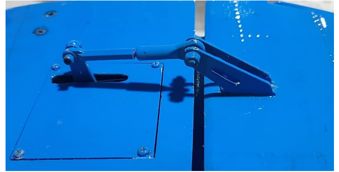
Above: elevators servos, servo arms and horns position with linkage.
