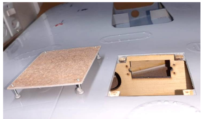
Above: servos fixation bases location on wing's ribs. Aileron (left) and flap (right).
