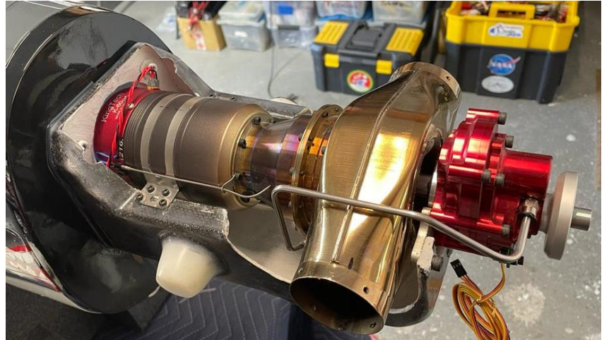
Above: turbine position on the carbon fiber turbine mount and lubrication tube position.
