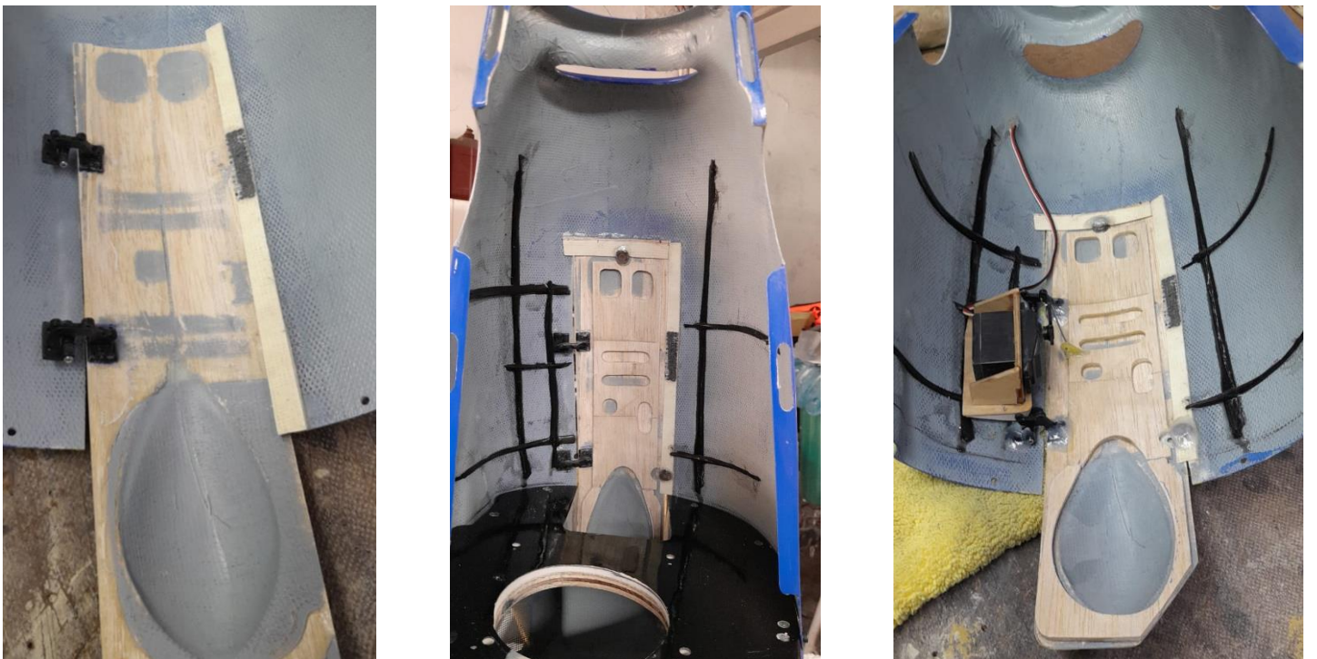
Above: bonding of front landing gear door hinges with balsa wood reinforcements and servo tray for opening and closing operation.
