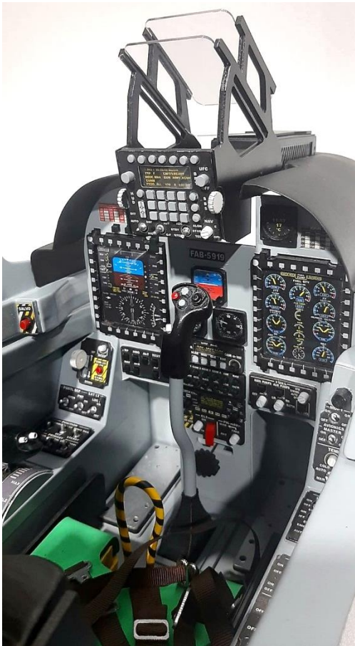
Above: detailed scale cockpit with front seat, instruments, stick, throttles and HUD.
