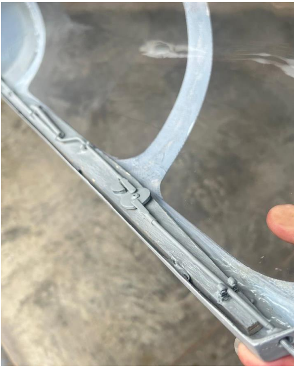
Above: opening and closing system for the canopy set (front part) with front latch.
