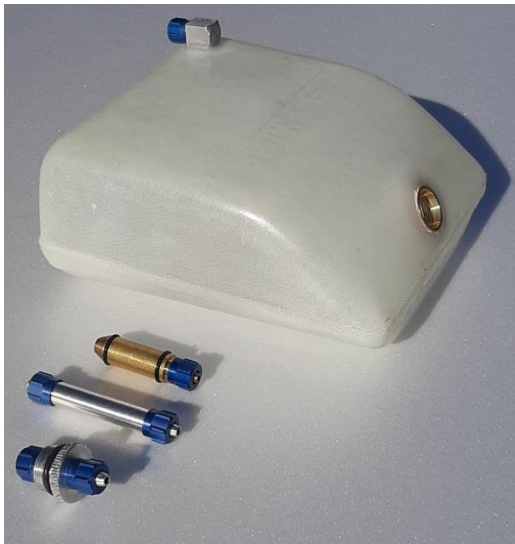
Above: fuel tank with Rio Jets nozzle and air vent installed and internal connections with cover.
