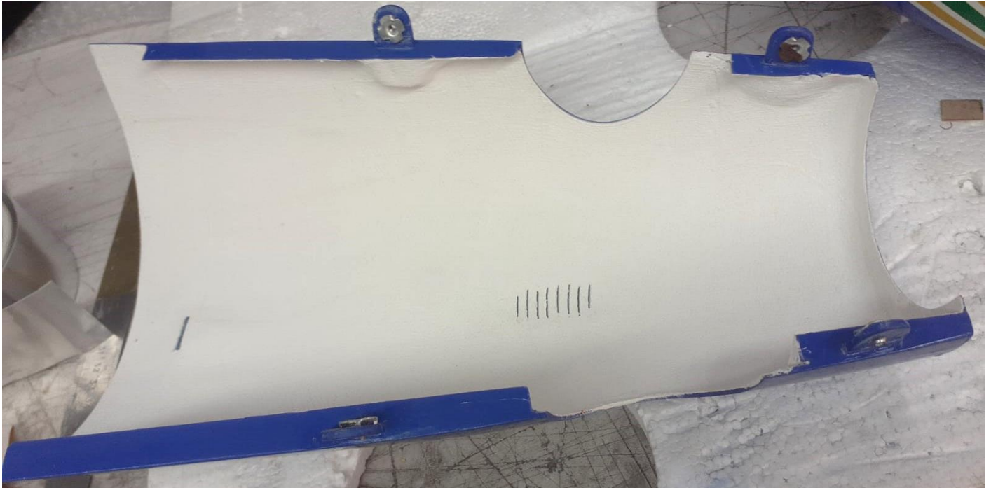
Above: upper cowling with 4 blind nuts 10-32 glued with epoxy and painted with water-based thermal protection paint with ceramic microspheres.
