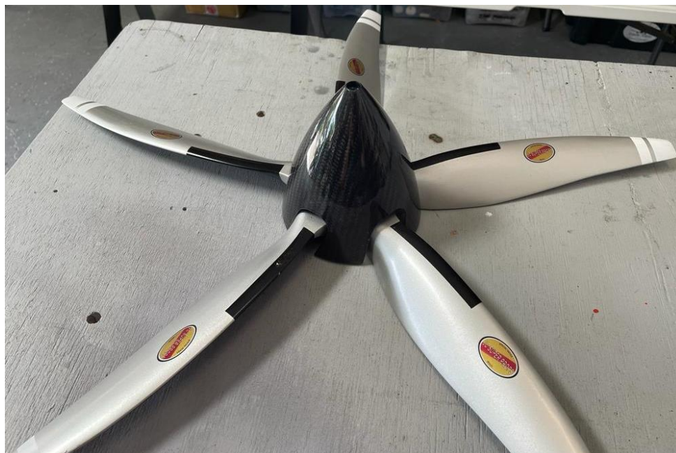
Above: spinner/propeller set ready and balanced. IMPORTANT: the spinner parts shall never touch the propeller.
