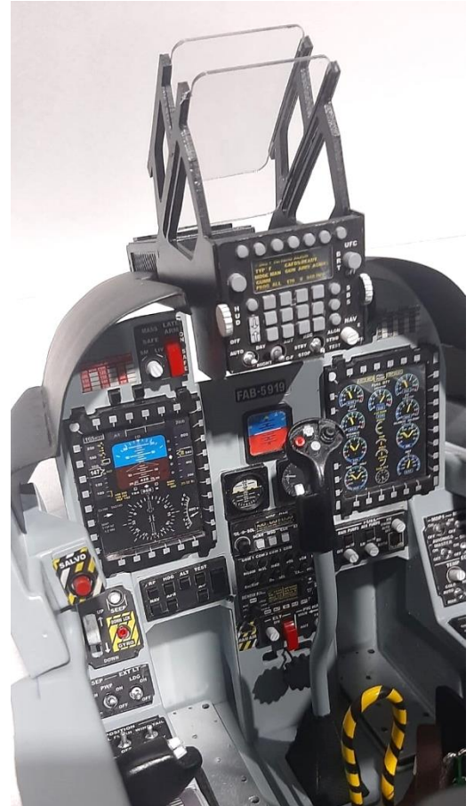
Above: detailed scale cockpit with front seat, instruments, stick, throttles and HUD.
