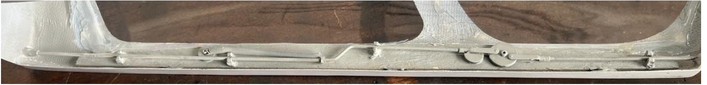
Above: opening and closing system for the canopy set with latches on the front and back.
