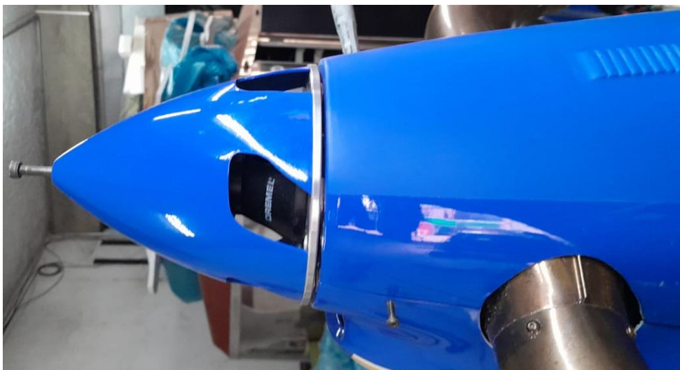
Above: alignment of the 2 parts of the cowling with the spinner and holes for the exhaust pipes.
