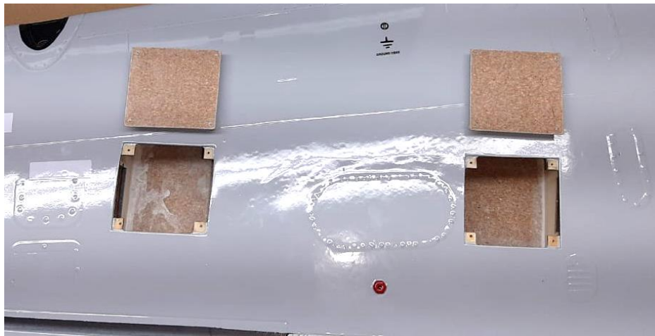
Above: servo compartment access covers location for ailerons and flaps servos and fixation holes on ribs.
