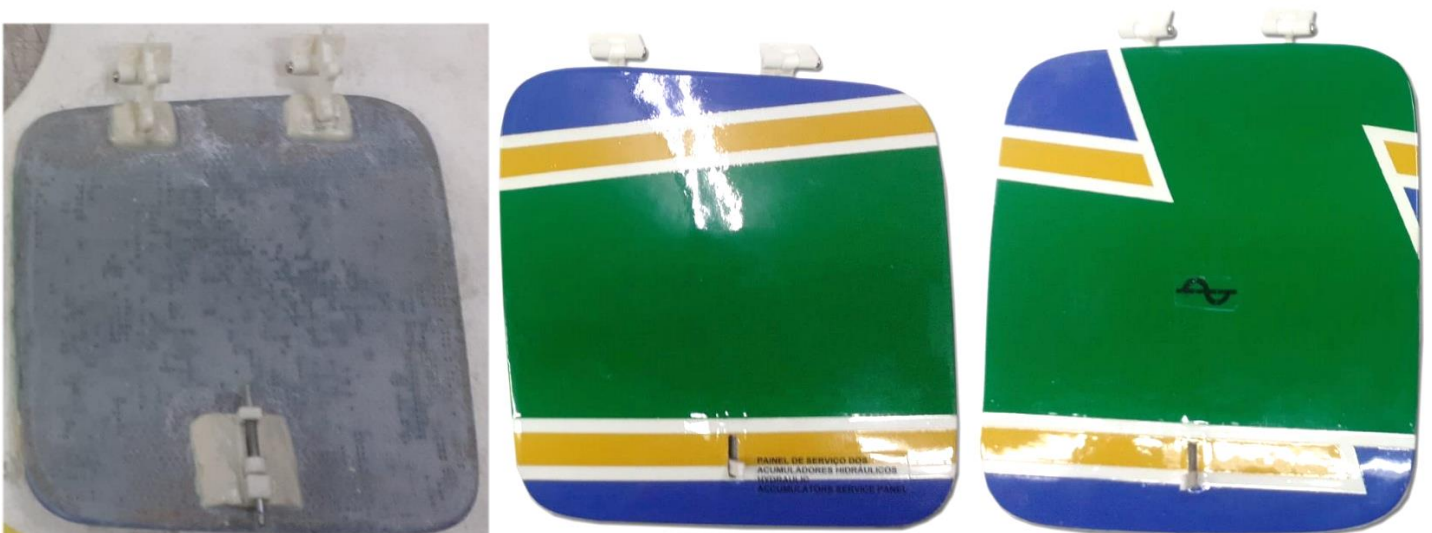
Above: door with installed hinges and latch seen by the inside (left) and outside (right).
