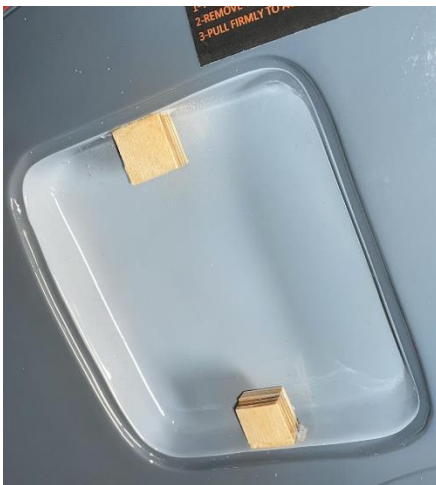
Above: wooden blocks glued in internal part of compartment (left), door in correct place (center) and screws for fixing the door to the fuselage (right).
