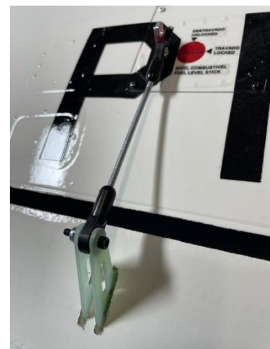
Above: aileron and flaps horns gluing process. Open slots (left), horns position with installed LED linkage (center) and glued horns on aileron command surface (right).
