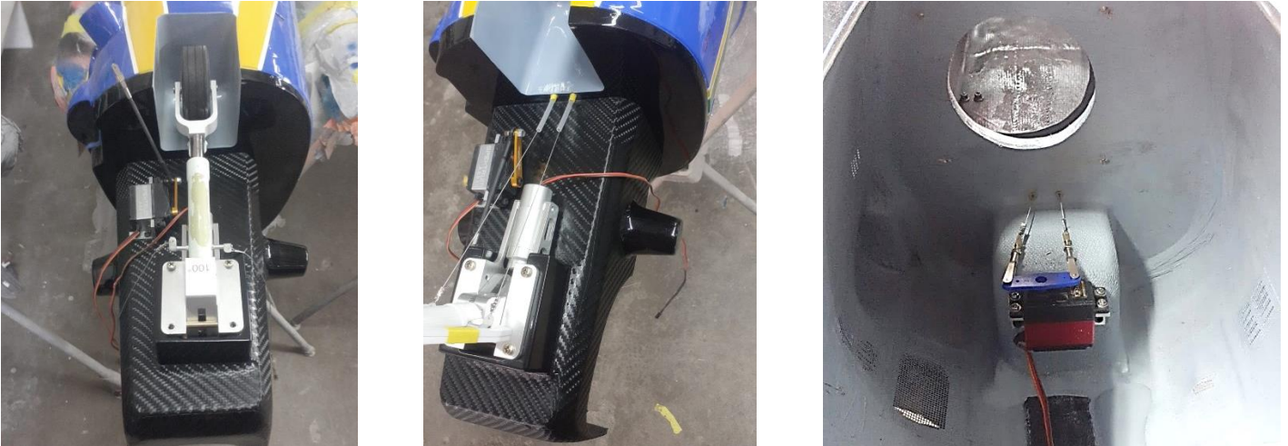
Above: front retract fixed to the turbine mount with steel pull-pull cables (left and center) and servo with pull-pull linkage for controlling the front wheel independent of the rudder servo (right).
