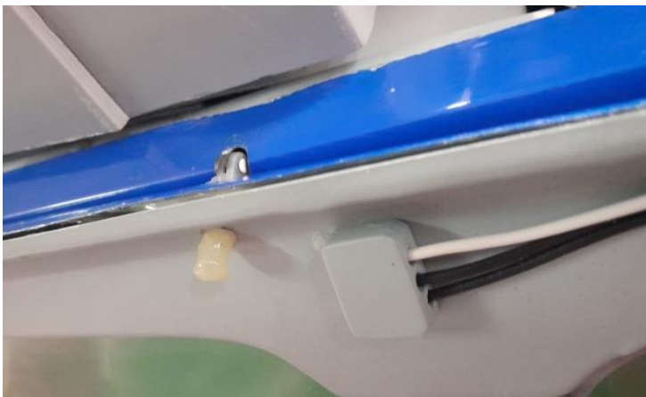
Above: details of the gluing of a canopy hinge inside the fuselage, through the scale cockpit (left) and the 2 installed hinges seen from the outside of the fuselage (right).
