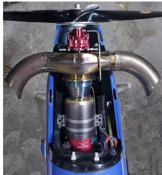
Above: cut exhausts position on turbine for realistic and scale appearance.
