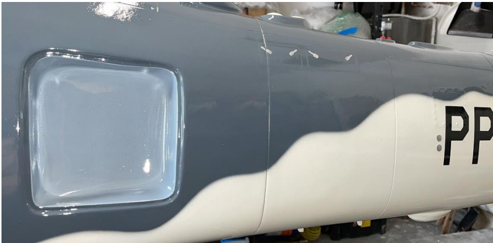
Above: the 2 fuselage sections joined after gluing and tightening the screws.
