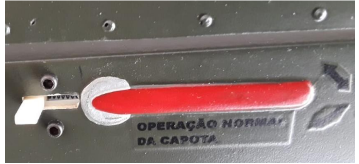
Above: lock position of the canopy / frame assembly on the fuselage.
