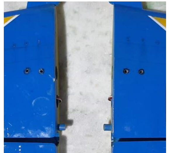
Above: position of the tube in the middle of the stabilizer and fuselage (left) and detail of the holes location for fixing the stabilizer halves in the stabilizer tube (right).
