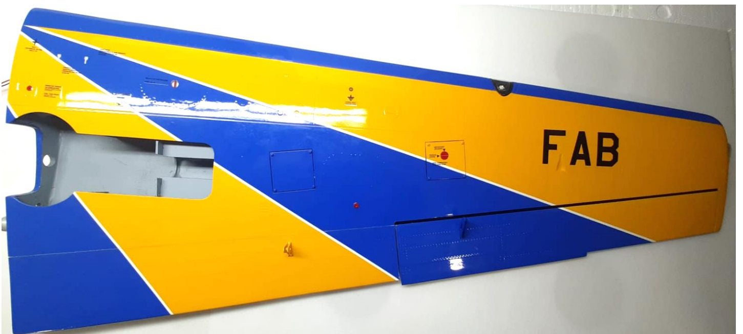
Above: horns positioned and glued to the left wing (note that the flap horns are straight and the aileron horns curved).
