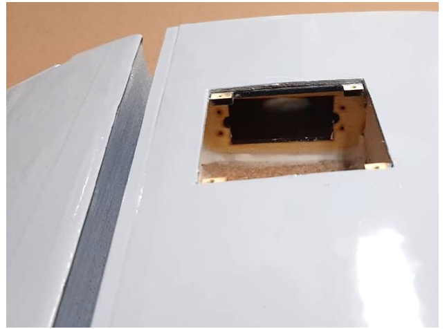
Above: elevator servo compartment access cover location (left) and servo fixation rib (right).
