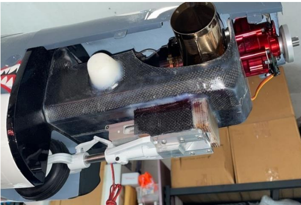
Above: upper cowling alignment with propwasher and exhausts holes.
