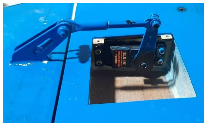
Above: elevators servos, servo arms and horns position with linkage.
