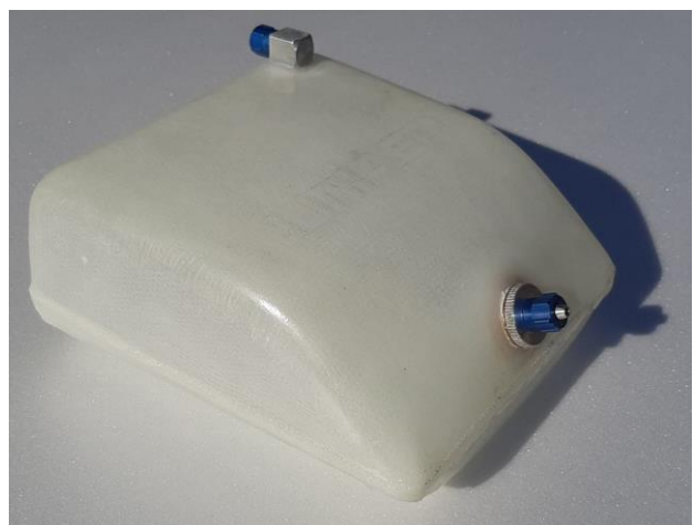
Above: fuel tank with Rio Jets nozzle and air vent installed and clunk assembly with extender and cover (left) and fully assembled fuel tank ready for installation on model airplane (right).
