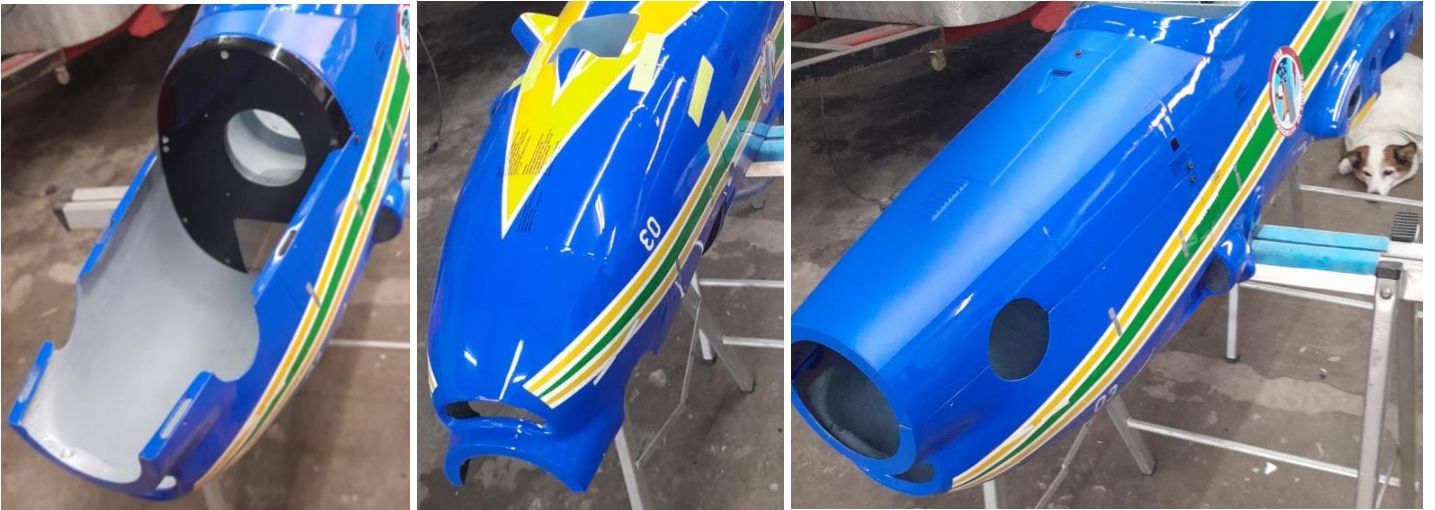
Above: lower cowling screwed to the fuselage in the correct alignment (left and center) and the 2 cowling parts already with holes for exhausts in the correct alignment (right).
