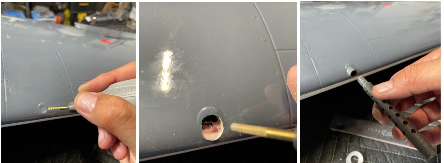
Above: hole opening for installing the machine gun replica close to the leading edge of the wing.
