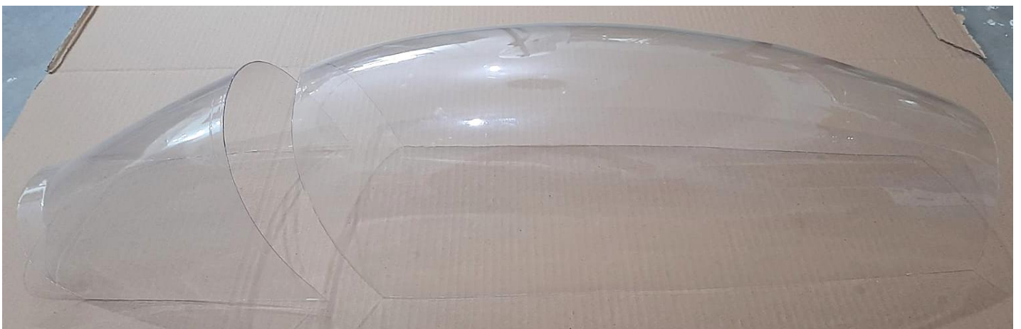
Above: correct desired shape of the 2 canopy parts after cut.
