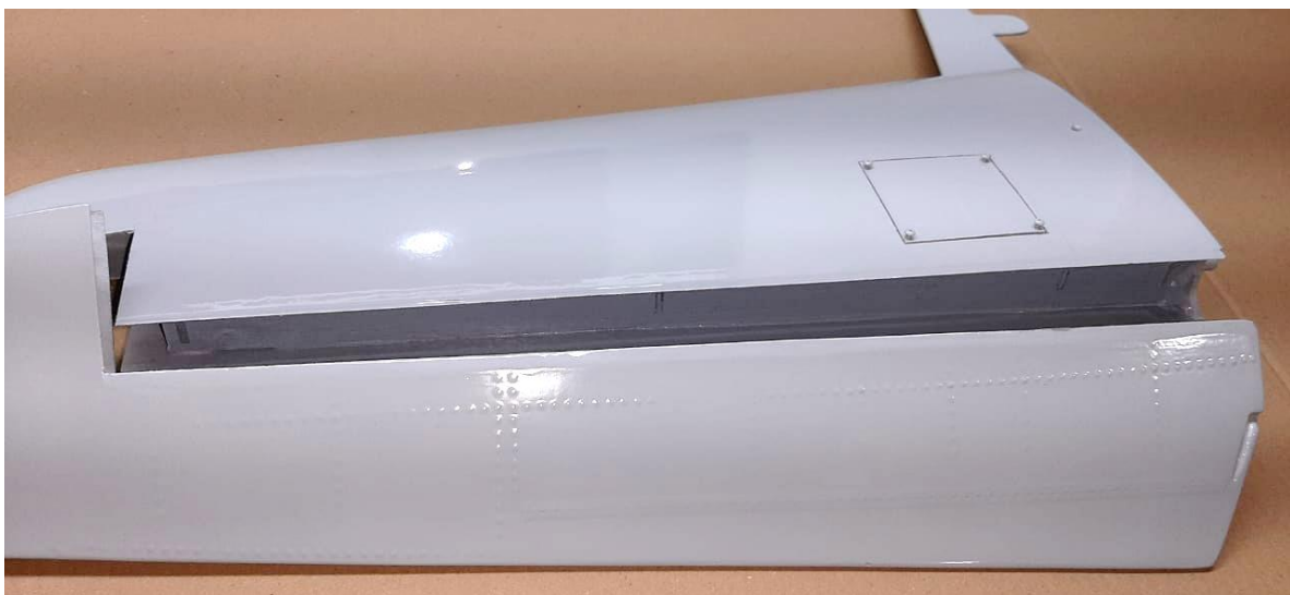
Above: gray areas (trailing edges) on stabilizer shall not be drilled or cut.
