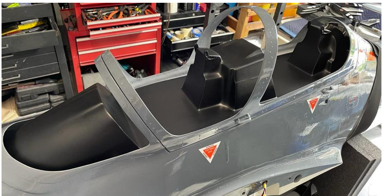
Above: stock simple cockpit fitted to the fuselage with canopy frame.
