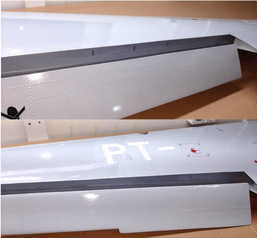
Above: gray areas (trailing edges) on ailerons and flaps shall not be drilled or cut.
