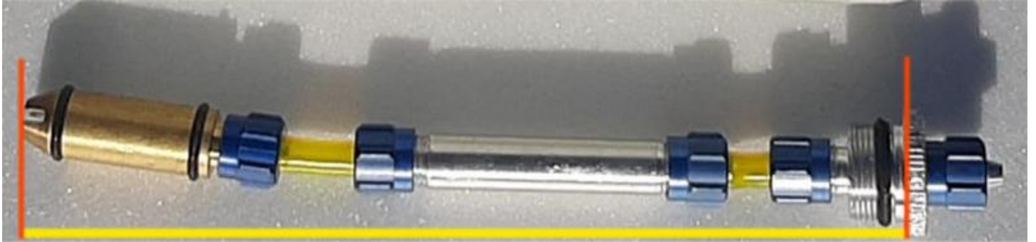
Above: total length of clunk assembly 16,5cm.
