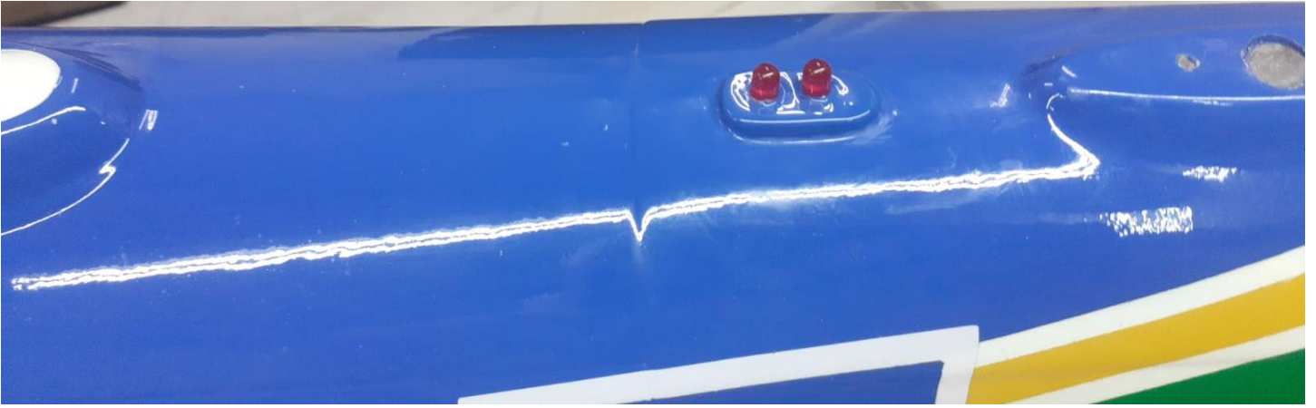
Above: definitive position of the red LEDs on the back of the fuselage after internal fixing of the board.
