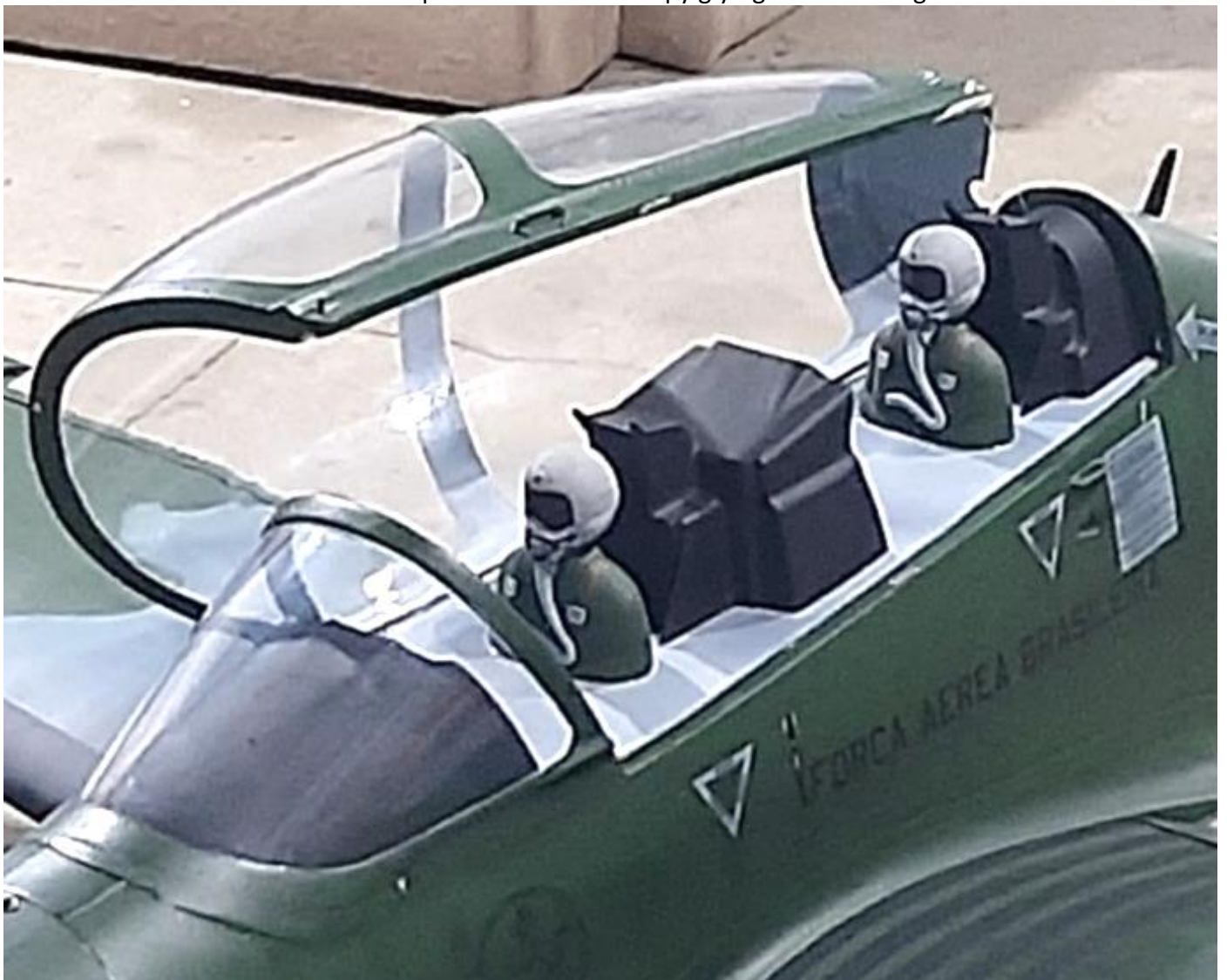
Above: front clear canopy glued to the fuselage and rear canopy glued to the canopy frame with side opening.
