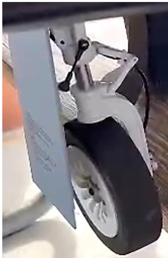
Above: right main landing gear and landing gear door connection made with a psuhrod and 2 ball links in the front part of the retract.
