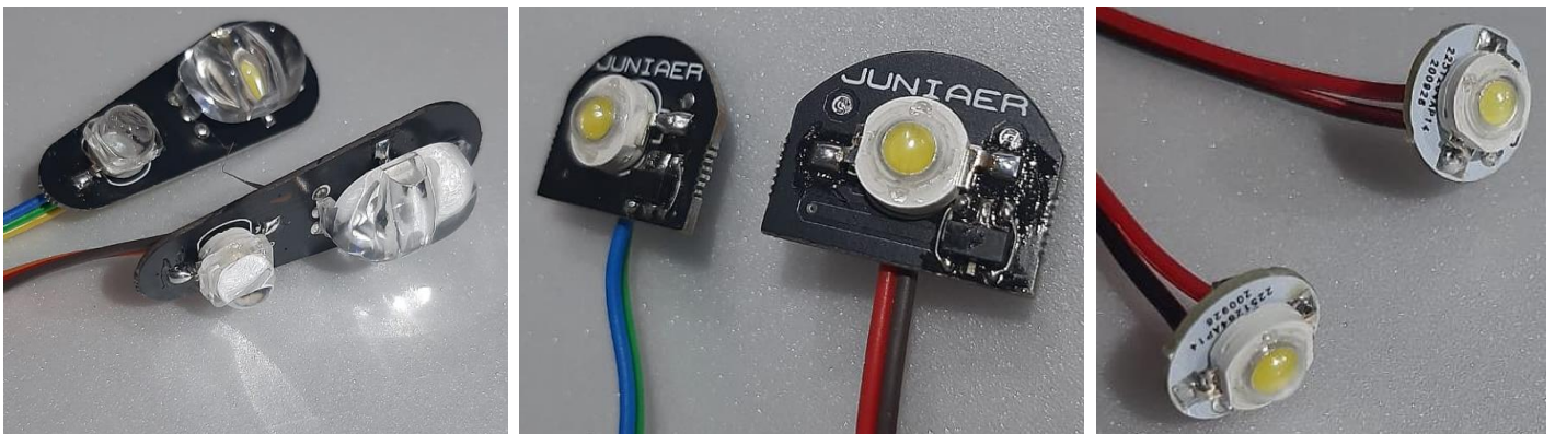
Above: wingtip boards with navigation lights and strobes (left), wing landing lights (center) and front landing gear landing lights (right).
