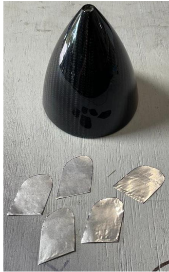
Above: spinner cut sequence to install the 5-blade propeller using equal shape adhesives.
