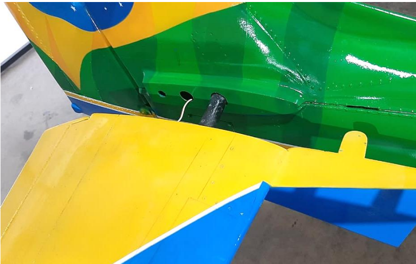
Above: position of the tube in the middle of the stabilizer and fuselage (left) and detail of the holes location for fixing the stabilizer halves in the stabilizer tube (right).
