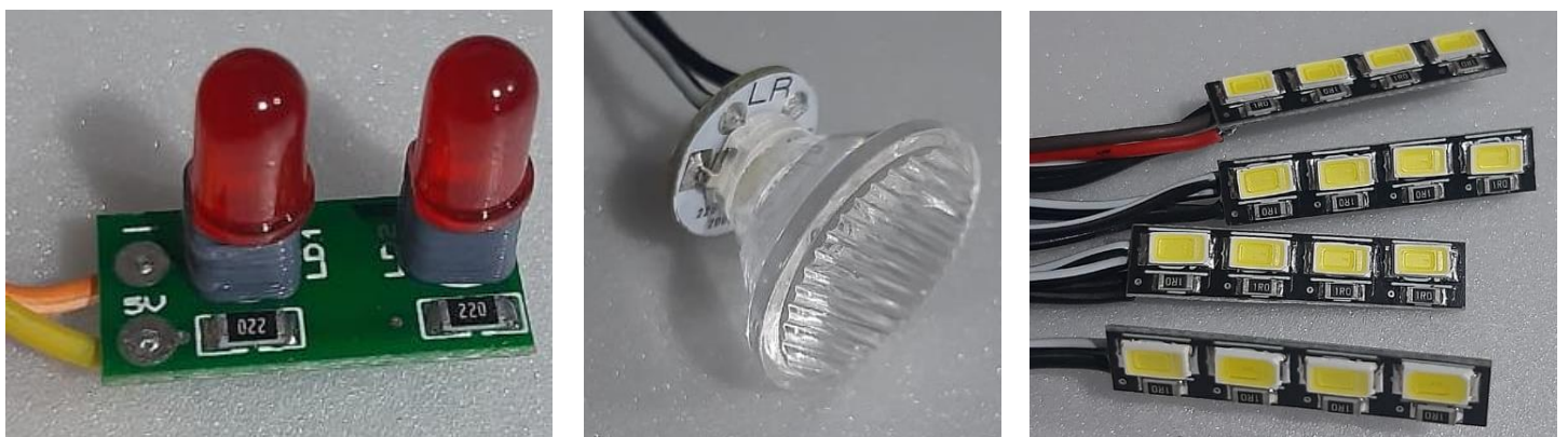
Above: fuselage dorsal beacon (left), fuselage intercept headlight (center) and vertical stabilizer formation lights (right)
