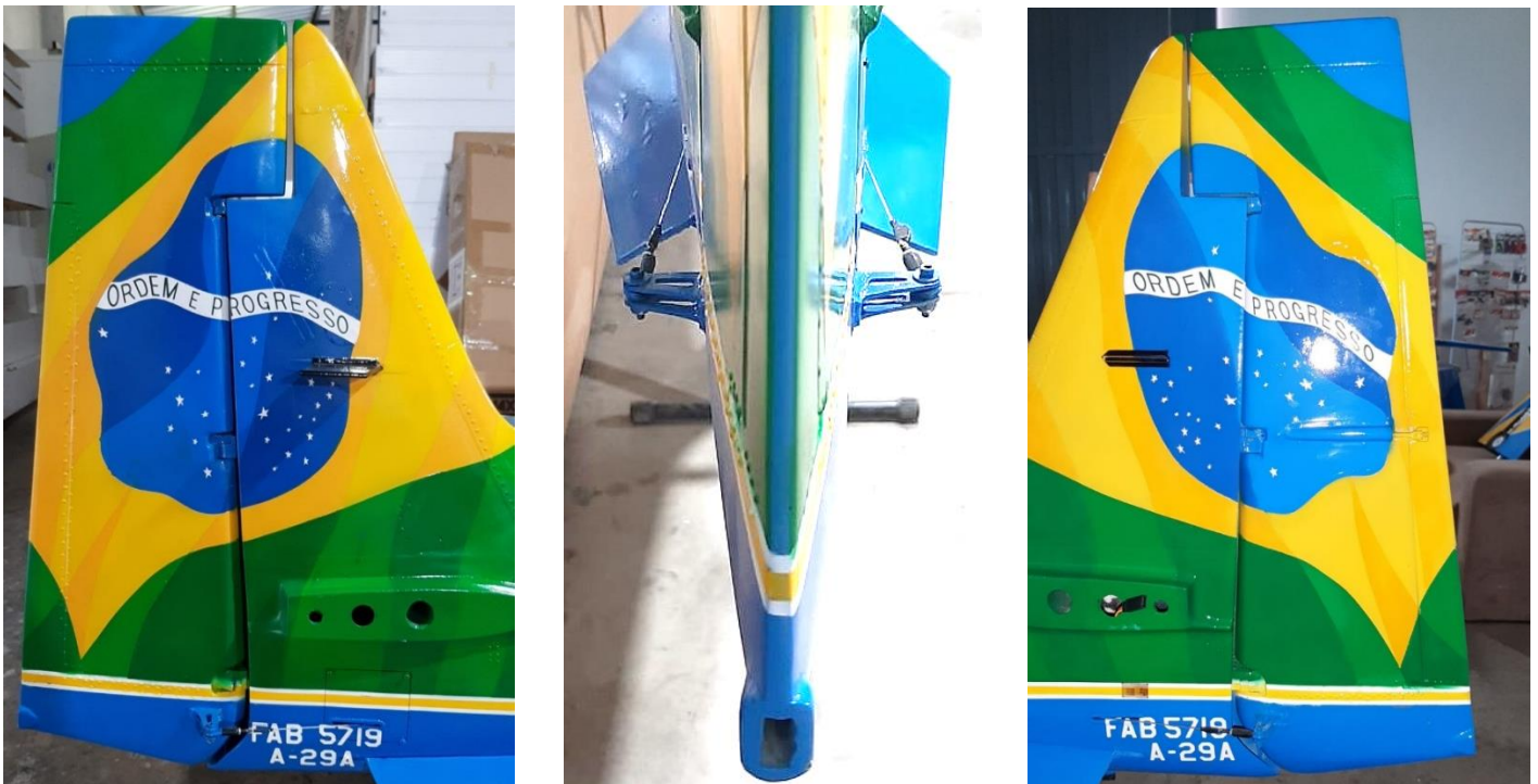
Above: pull-pull steel cables exits with Dubro heavy duty 4-40 ball links fixed on control horns with 4-40 screws and parlock nuts on both sides of the fuselage and rear view.
