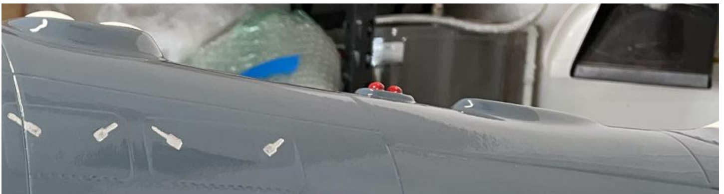
Above: position of the LED replicas on the fuselage back that must be cut and drilled with a 5mm drill.
