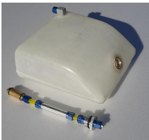
Above: fuel tank with Rio Jets nozzle and air vent installed and clunk assembly with extender and cover (left) and fully assembled fuel tank ready for installation on model airplane (right).
