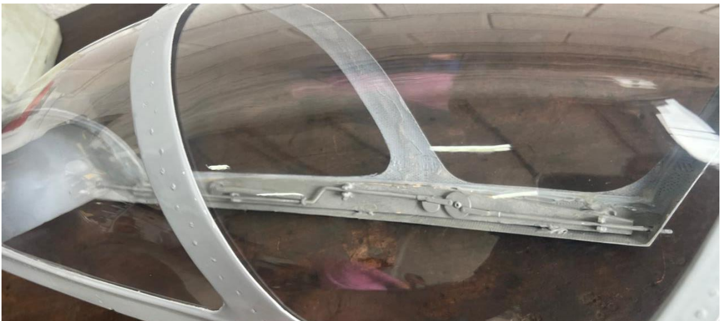
Above: opening and closing system for the canopy set with latches on the front and back.
