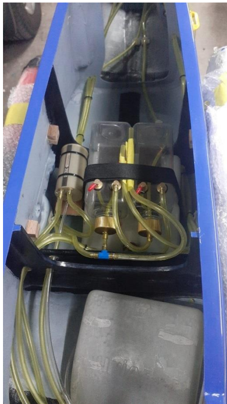
Above: 2 500ml smoke fluid tanks installation above the rear fuel tank (left) and UAT on right also above the rear fuel tank (center and right).
