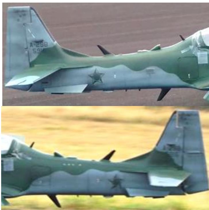
Above: A-29 Super Tucano 80cc Juniaer profile showing antennas and fins positions.
