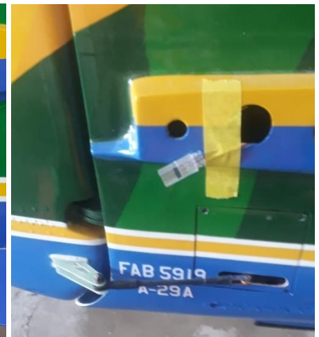
Above: rudder servo position inside the fuselage (left), servo arm linkage (center) and complete linkage with double HD horns(right).
