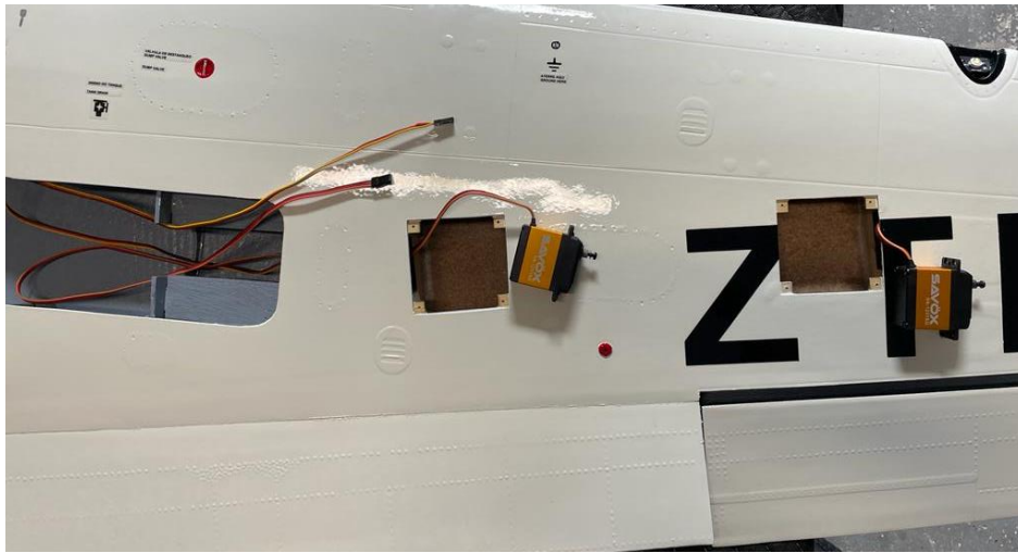
Above: thread and extensions passing process on wing with the servos.
