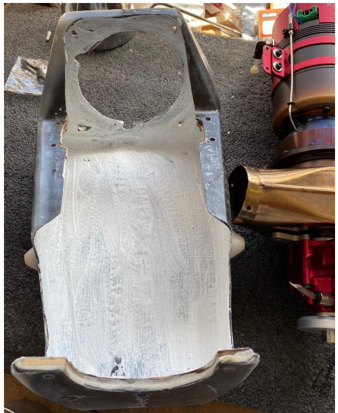
Above: application of 1 coat of thermal protection paint in the turbine carbon mount.
