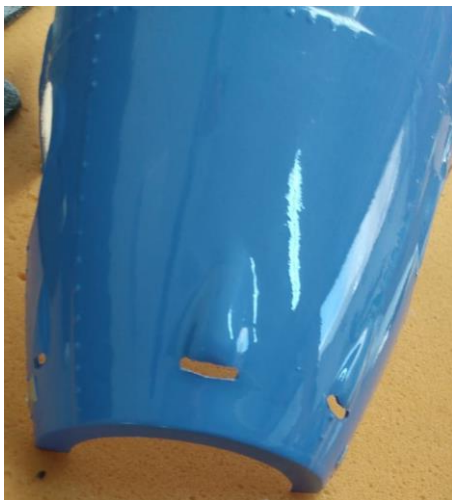
Above: 3 holes in the 3 reliefs of the upper cowling, on the front, to increase the cold air flow.
