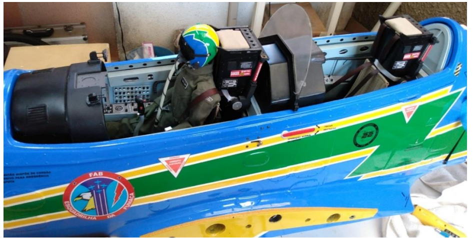
Above: Inner canopy frames installed (left) and all cockpit parts (front cockpit, rear cockpit, cockpit divider, rear part and inner frames installed (right).
