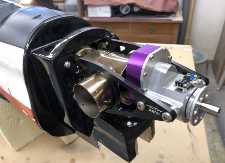
Above: Xicoy X45 position at the firewall without exhausts (left) and with exhausts (right).
