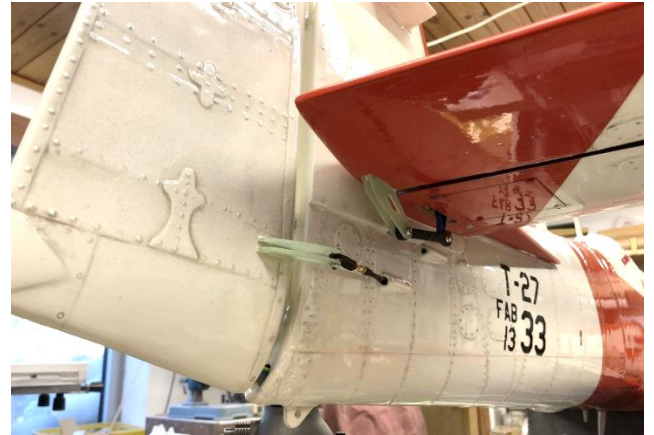
Above: elevator servo, servo arms and horns position and pull-pull steel cables exit with rudder double horn.
