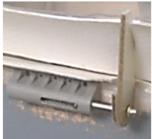
Above: locking the canopy assembly / canopy frame inside the fuselage.
