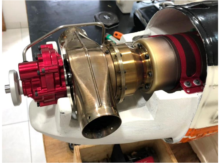
Above: turbine position and turbine mount on the fire wall (left) and turbine mount painted with thermal protection paint (right).
