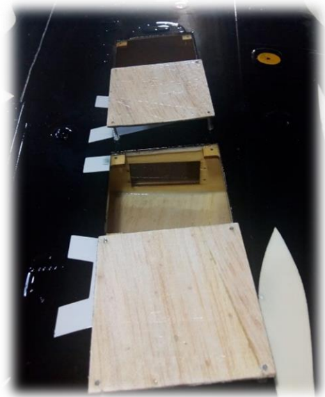
Above: servo compartment access covers location for ailerons and flaps servos and fixation holes on ribs.
