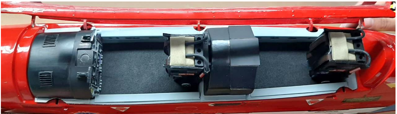
Above: in case of internal hinges for canopy/frame side opening it's necessary to open slots on the cockpit to allow the actuation of hinges and locks.
