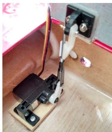
Above: micro servo installed with horn and linkage for mechanism acting.
