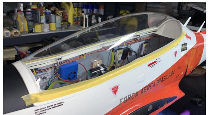
Above: clear canopy cut and ready to glue (left) and glued and in place with masking tape.
