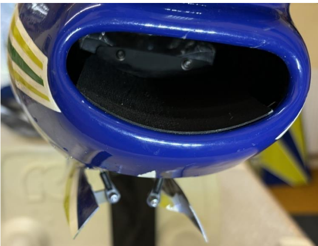
Above: Wren 44 turbine installed in the firewall with exhausts.
