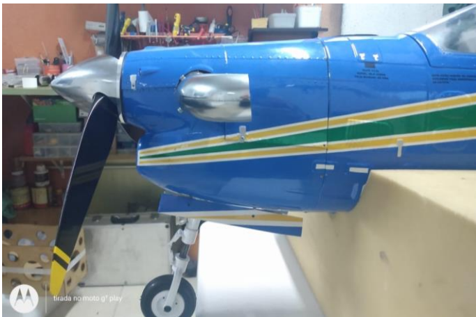
Above: correct alignment of the nose cowling with the propeller and spinner assembly and turbine exhausts.
