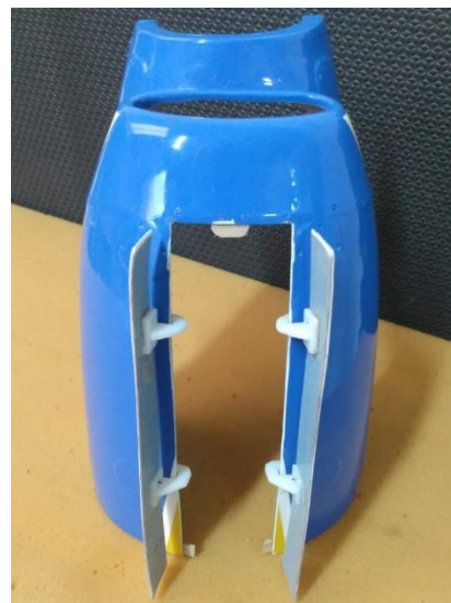
Above: hinged with doors and compartments hinges, the two front doors of the front landing gear to the lower engine cowling.
