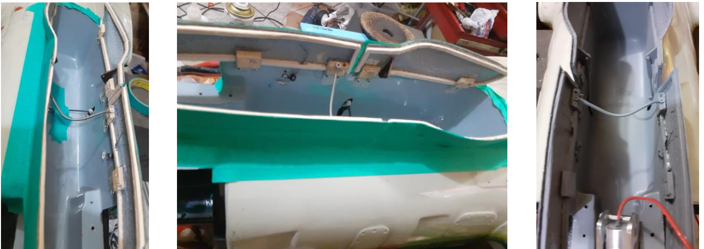
Above: installation of a mechanism for opening and closing the doors of the front landing gear.
