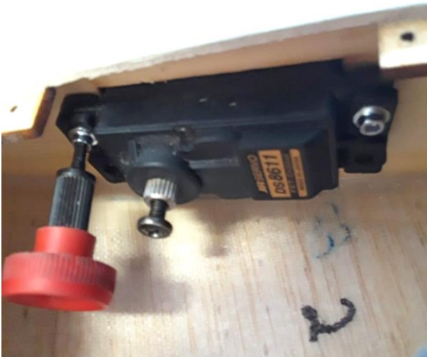
Above: short screwdriver and correct position to screw the wing's servos.
