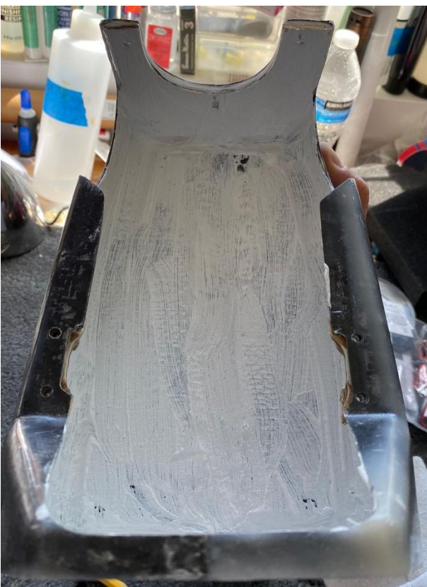
Above: application of 1 coat of thermal protection paint in the turbine carbon mount.
