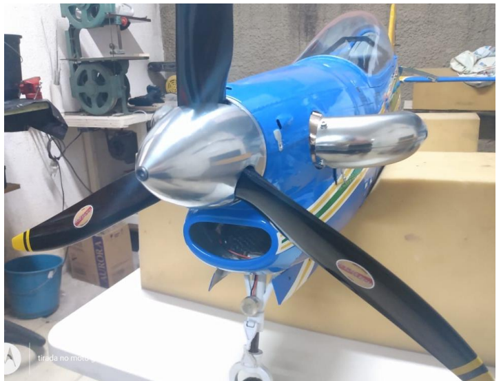
Above: Correct alignment of the nose cowling with the propeller and spinner assembly and turbine exhausts.
