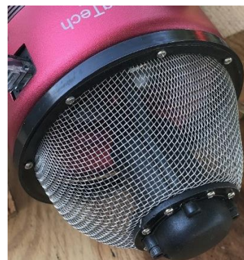
Above: it is recommended to install a FOD screen to protect the air intake of the turbine in order to avoid absorption of solid particles by the turbine.
