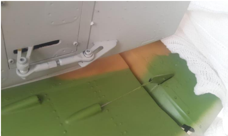
Above: elevator servo, servo arms and horns position and pull-pull steel cables exit with rudder double horn.
