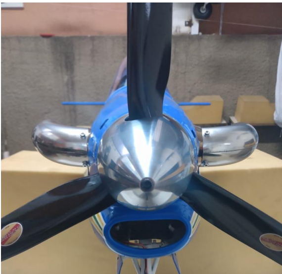
Above: Correct alignment of the nose cowling with the propeller and spinner assembly and turbine exhausts.
