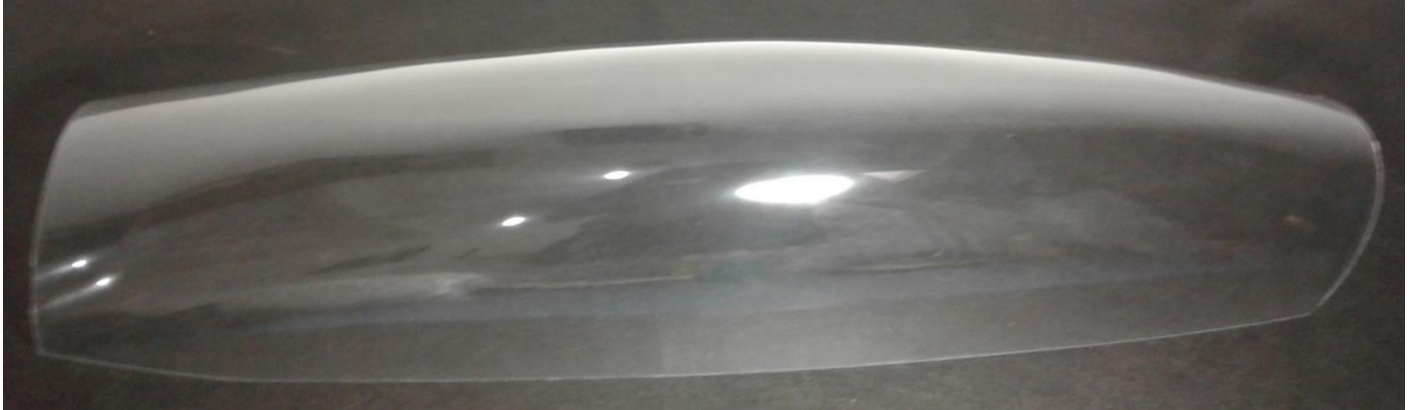
Above: correct desired shape of the clear canopy after cutting.
