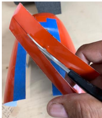
Above: cutting process of the lower engine cowling and the 4 landing gear doors of the front landing gear.
