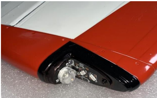
Above: correct locations for fixing wingtip light boards (left) and landing lights (right).
