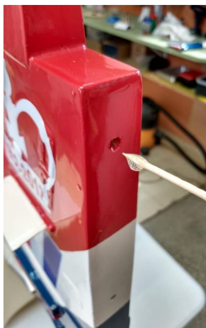
Above: rudder hinge points epoxy gluing sequence.
