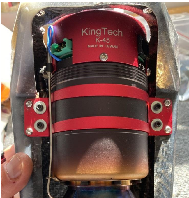
Above: position of the 4 turbine horizontal fixing screws on the carbon turbine mount (left) and the 3 turbine vertical fixing screws on the carbon turbine mount (right).
