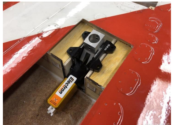
Above: hardwood blocks added to the retracts bases (left) and Electron retract on base (right).
