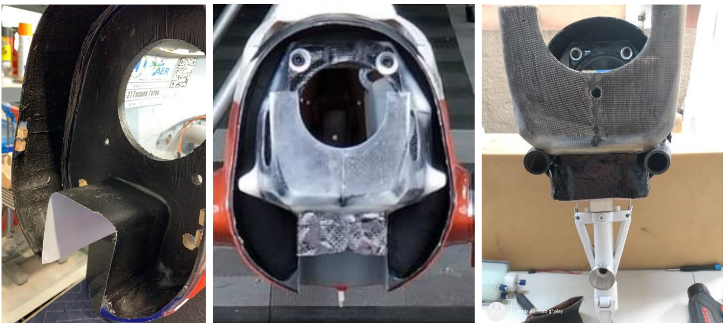
Above: carbon fiber turbine mount position on the firewall.
