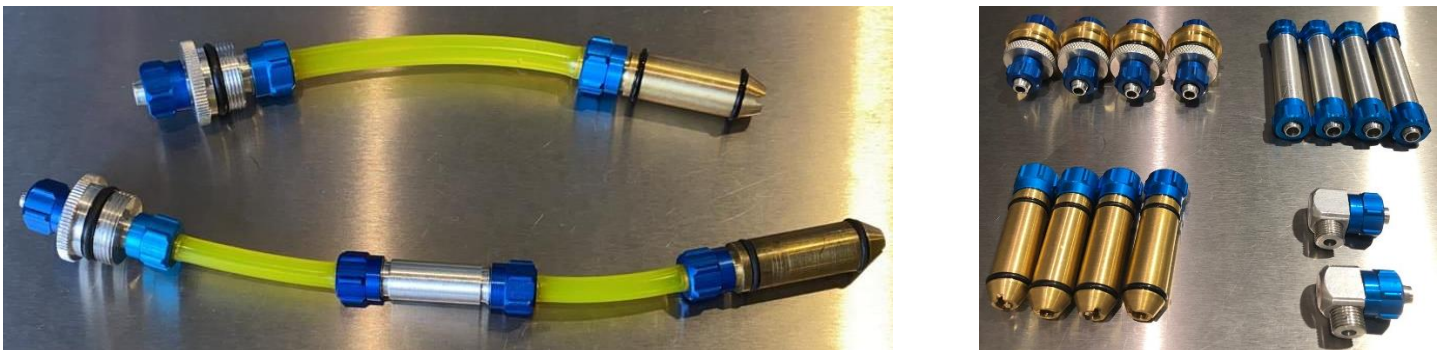
Above: clunk mounted without extender (above) and with clunk extender (below) to prevent hose bending (left) and complete connections including vent manufactured by Rio Jets (right).
