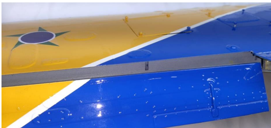
Above: gray areas (trailing edges) on ailerons and flaps shall not be drilled or cut.
