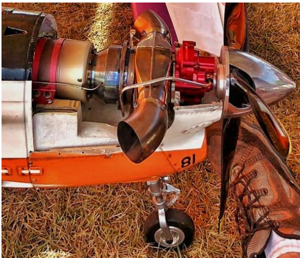
Above: turbine installed with the lubrication tube lowered to allow the installation of the upper cowling and exhausts with a 90 degrees outlet indicated for the T-27 Tucano 45TP.
