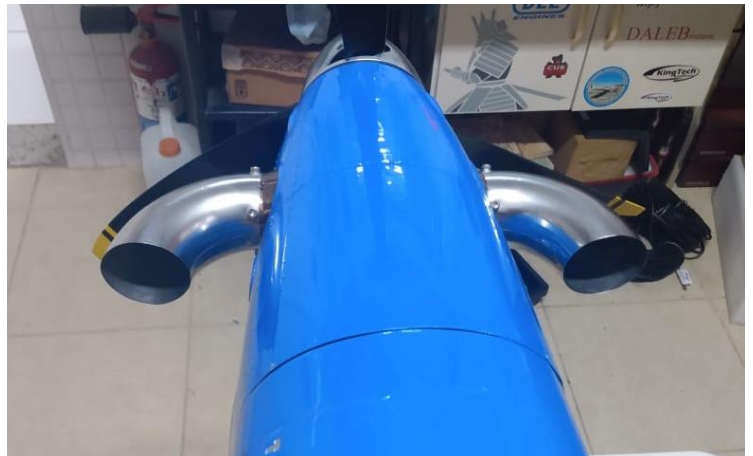
Above: correct alignment of the nose cowling with the propeller and spinner assembly and turbine exhausts.
