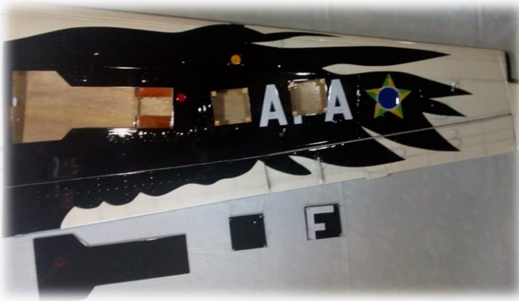
Above: servo compartment access covers location for ailerons and flaps servos and fixation holes on ribs.
