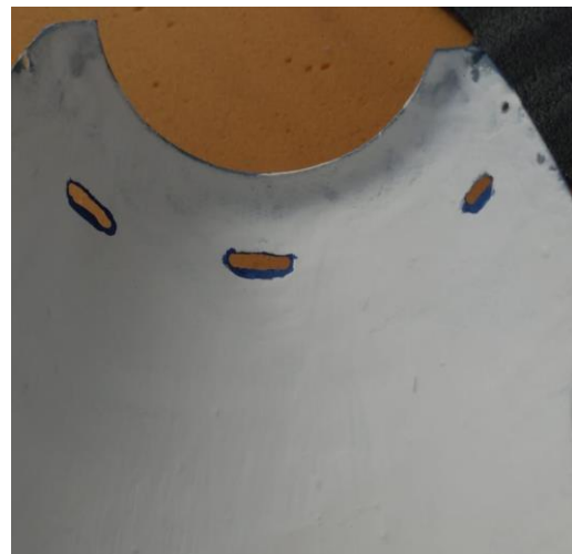
Above: 3 holes in the 3 reliefs of the upper cowling, on the front, to increase the cold air flow.
