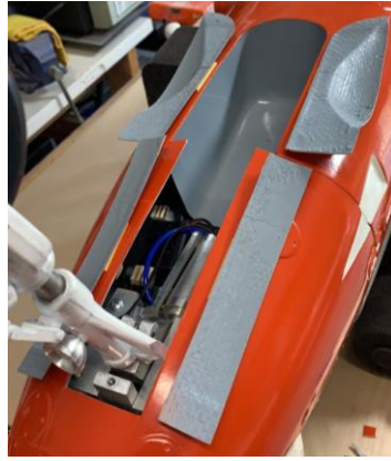
Above: the 4 landing gear doors of the front landing gear cut out (left) and their positions (center and right).
