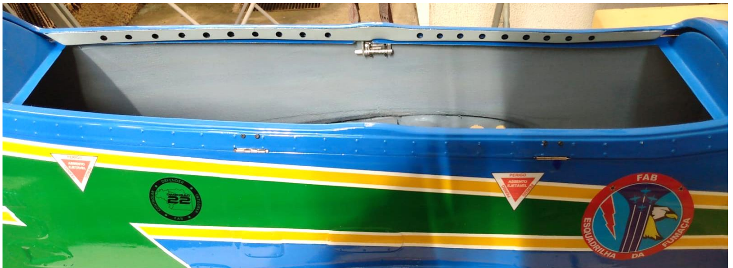
Above: position of the inner frame of the canopy frame.
