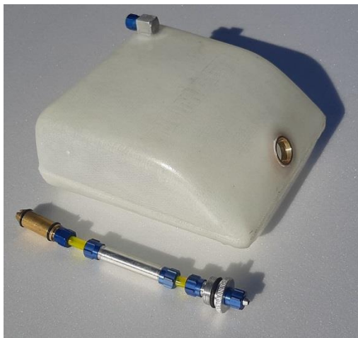
Above: tank with Rio Jets nozzle and vent installed and clunk set with extender and cap (left) and ready to install and fully assembled fuel tank (right).
