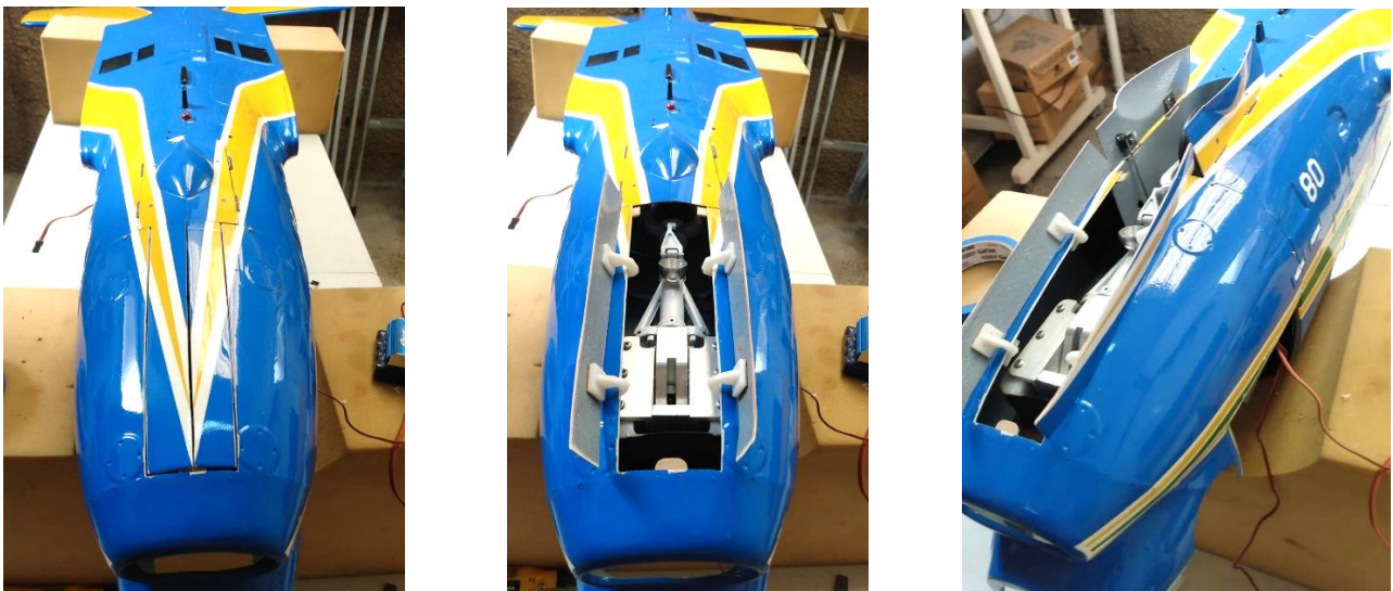
Above: the 4 front landing gear doors closed (left) only the front ones open (center) and all doors open (right).
