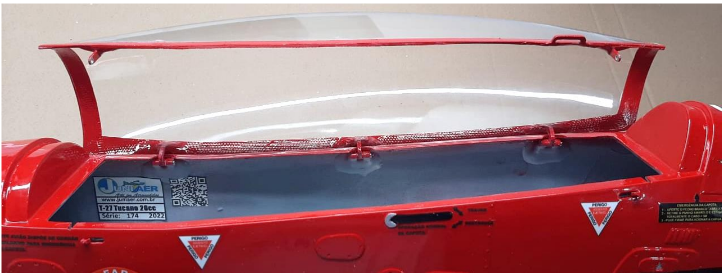
Above: canopy/canopy frame assembly with double locking, using 2 locks.
