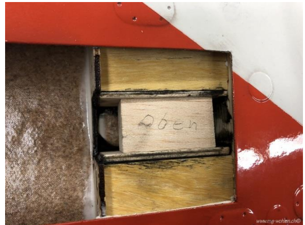
Above: hardwood blocks shaped to fit the retracts bases (left) and gluing process (right).
