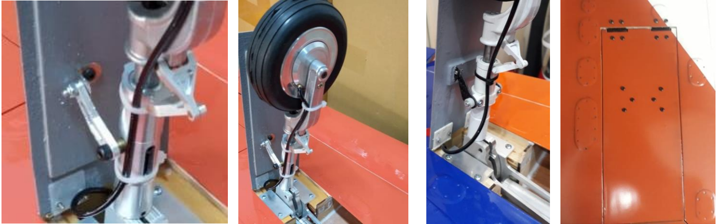
Above: detail of the articulated supports attachment to the external landing gear door of the external landing gear and closed external landing gear door (right).
