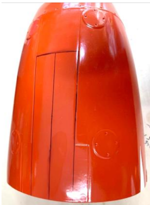
Above: fixed with Dubro hinges, the two front landing gear doors of the front landing gear in the lower engine cowling (left) and the two rear doors of the front landing gear in the fuselage (right).
