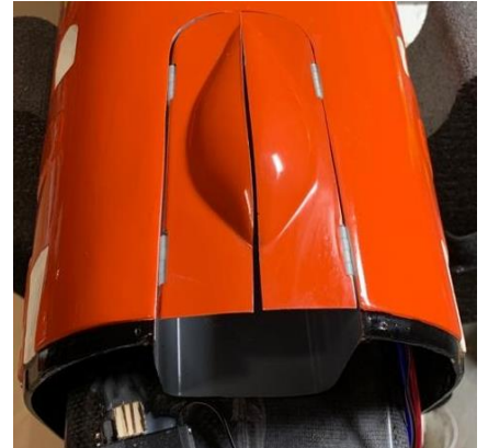
Above: fixed with Dubro hinges, the two front landing gear doors of the front landing gear in the lower engine cowling (left) and the two rear doors of the front landing gear in the fuselage (right).
