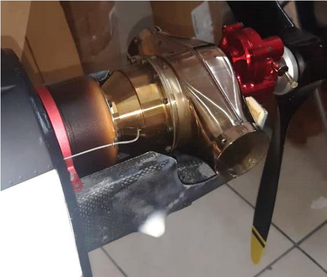
Above: turbine position and turbine mount on the fire wall (left) and turbine mount painted with thermal protection paint (right).
