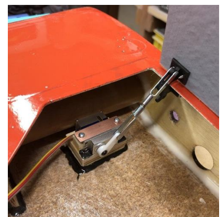
Above: door compartment hinges and micro servo installed with linkage.
