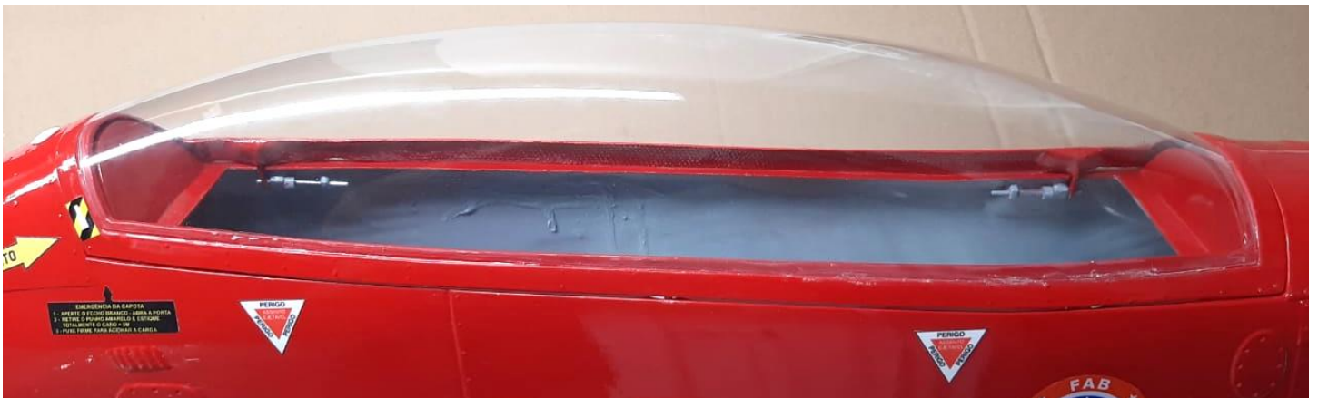
Above: canopy/canopy frame assembly with double locking, using 2 locks.
