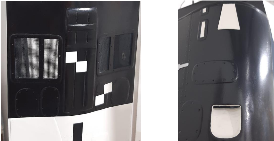
Above: openings in the lower part of the fuselage (left) and in the front part of the fuselage (right) for air intake by the turbine and cooling.
