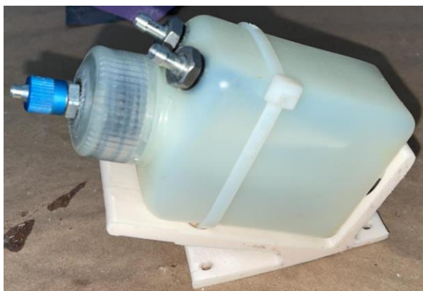
Above: example of UAT to be used between the fuel tank and the turbine fuel pump. The UAT must be positioned inclined at 45° in order to eliminate air bubbles from the fuel line and one of its upper connections is intended to supply the tank(s) through a hose with a plug.
