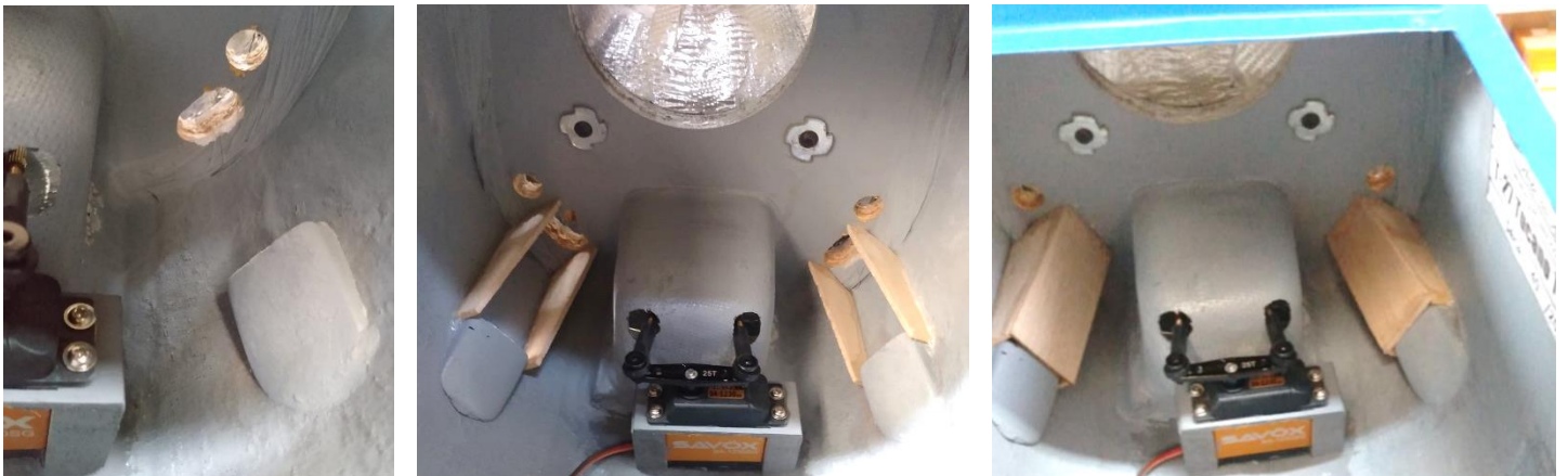
Above: openings in the lower front part of the fuselage for directing hot air from the turbine compartment out of the model aircraft by channeling the air through the firewall.
