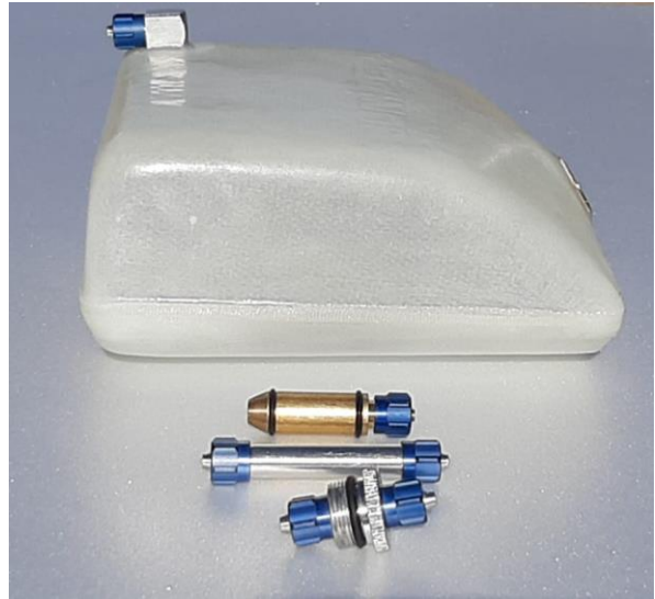
Above: tank with Rio Jets nozzle and vent installed and internal connections with cap.
