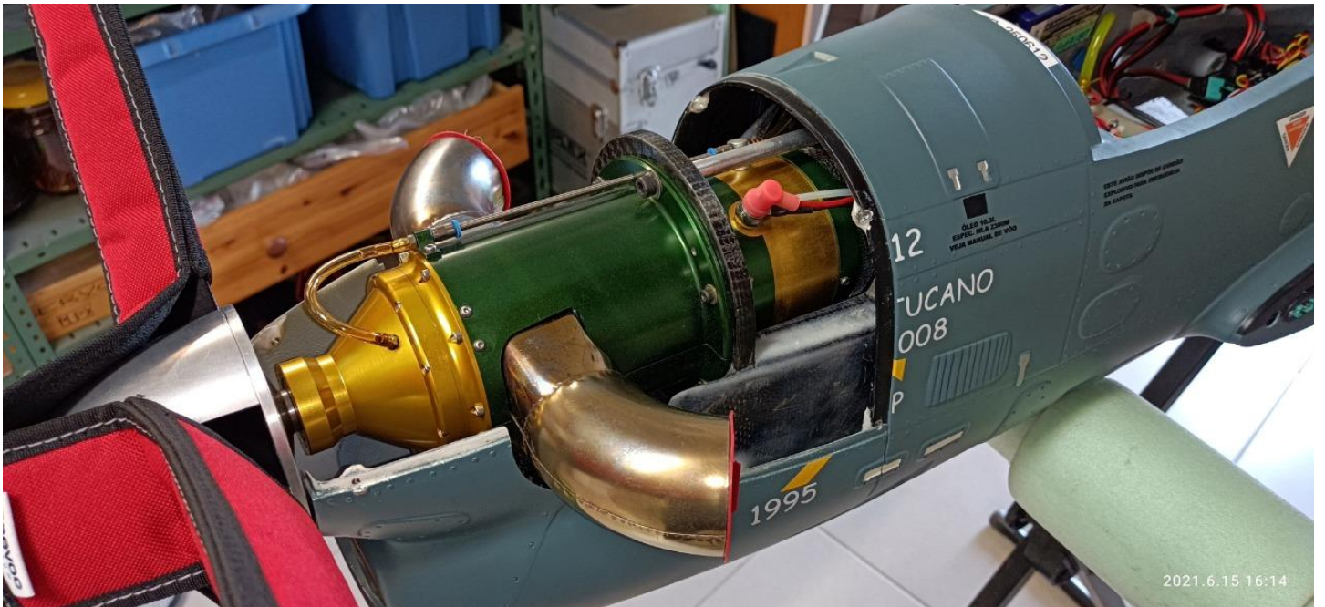
Above: Wren 44 turbine installed in the firewall with exhausts.
