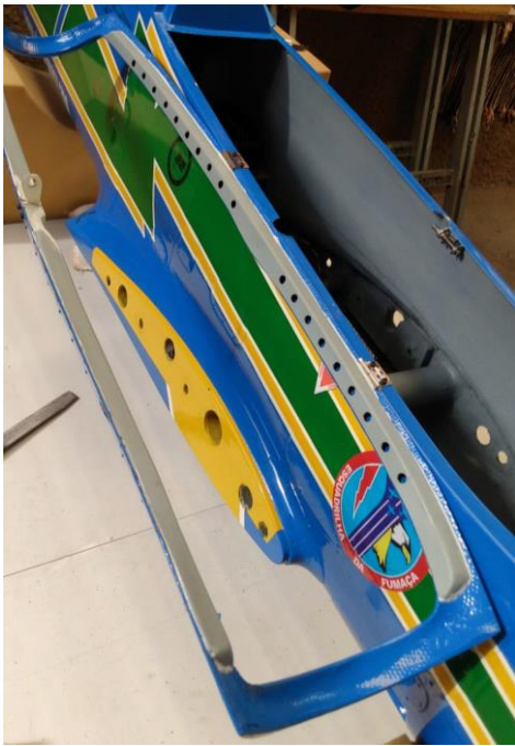
Above: Inner canopy frames installed (left) and all cockpit parts (front cockpit, rear cockpit, cockpit divider, rear part and inner frames installed (right).
