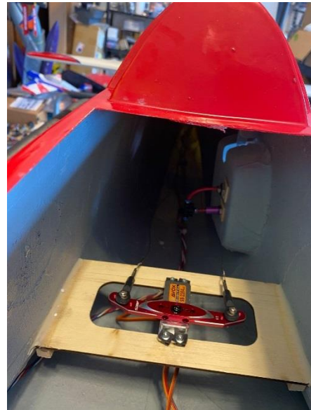
Above: stock servo tray positioned on inferior part of the fuselage to allow rudder servo instalation with Flávio scale cockpit.
