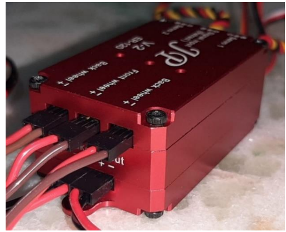
Above: JP ER-150 V2 controller with brakes showing retracts connections on upper side and brakes outputs on lower side. Note the correct polarity of wires as written at controller case.
