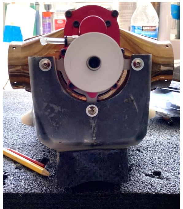
Above: position of the 4 turbine horizontal fixing screws on the carbon turbine mount (left) and the 3 turbine vertical fixing screws on the carbon turbine mount (right).
