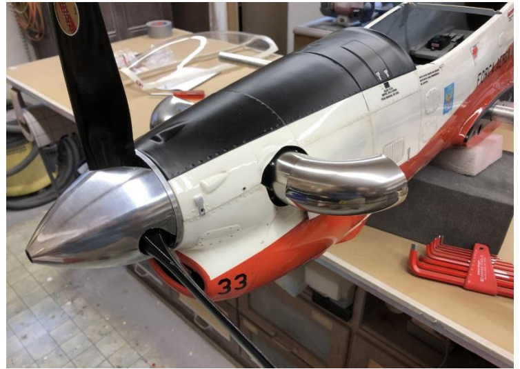
Above: Xicoy X45 with installed tachometer (left) and final position with exhausts, cowling, propeller and spinner (right).
