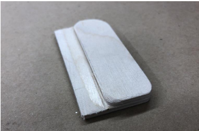
Above: hardwood blocks shaped to fit the retracts bases (left) and gluing process (right).
