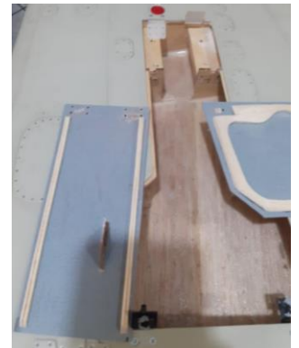
Above: landing gear door set (left) and main landing gear doors cut and reinforced (center and right).
