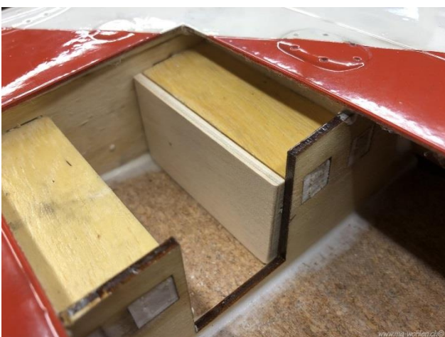
Above: hardwood blocks added to the retracts bases (left) and Electron retract on base (right).
