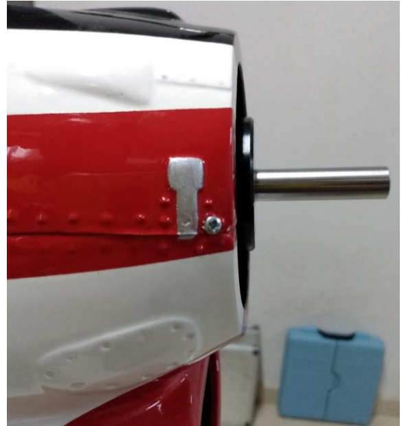
Above: installation of the lower cowling with the cutouts for the exhausts with the KingTech K-45TP turbine (left) and parallel alignment of the engine axis / fairing (right).
