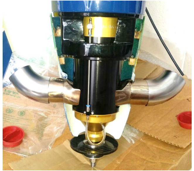
Above: T-27 Tucano 45TP firewall with specific firewall drilling for Wren 44 turbine (left) and Wren 44 turbine installed in the firewall with exhausts (right).
